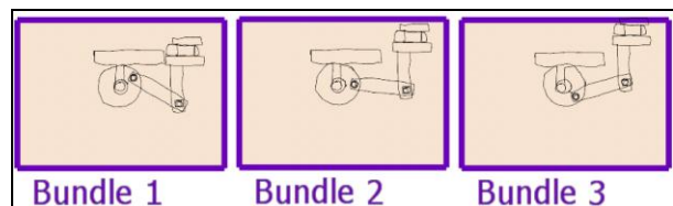
Figure 8: A device for re-training precision finger movements. The palm rests on the top with the finger stuck through a “key”. The up and down movement simulates typing.
