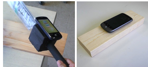
Figure 4: A smart phone put on a bar of a covered saw (left) and a smart phone put on a wood piece like a plane (right).
